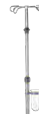
I.V.Pole stainless steel Ø 25 / 18 mm, one-hand height-adjustable 1070-1660 mm, 4 hooks, max. 2 kg 84,4 lbs/hook, glass and holder
